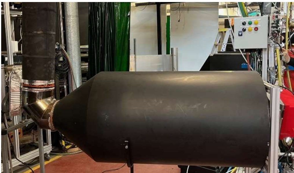
Figure 36 Schematic diagram (a) and photo (b) of the confined firing apparatus with a package burner.
