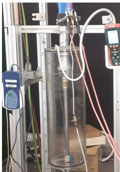
Figure 11: Enclosure for measurement/control of aeration for the AN burner.
