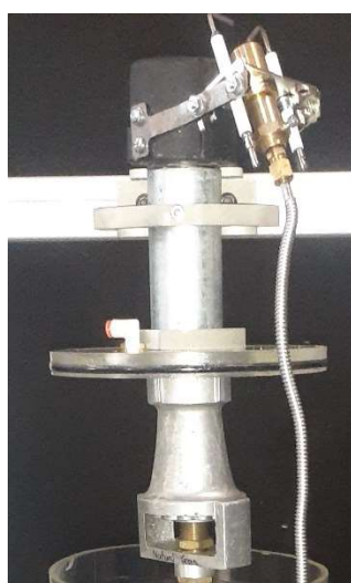
Figure 10: AN burner with pilot assembled.
