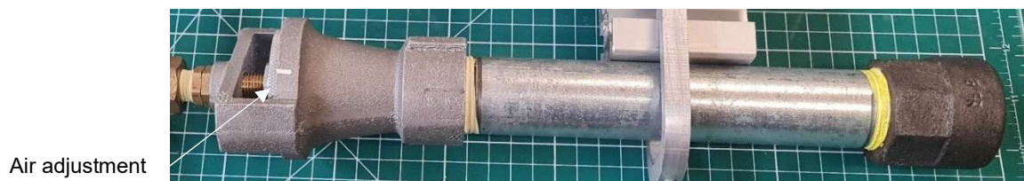
Figure 1 The FR 8 nozzle with air inlet closed
