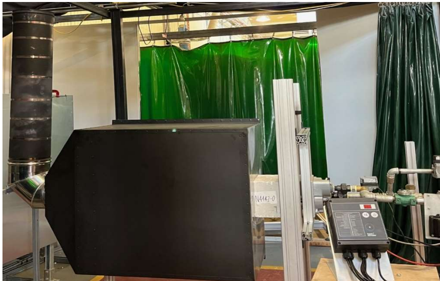
Figure 37 Schematic diagram (a) and photo (b) of the confined firing apparatus with a high-velocity nozzle-mix burner.
