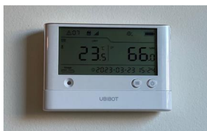
Figure 2 UbiBot WS1 Pro 2.4GHz temperature and relative humidity logger
