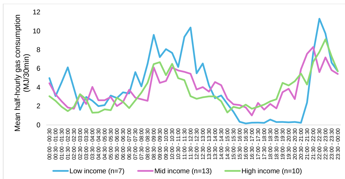
Figure 39 Comparison of diurnal variations of mean half-hourly gas consumption in low, mid and high annual income groups on days with a daily mean outdoor temperature of 11 °C
